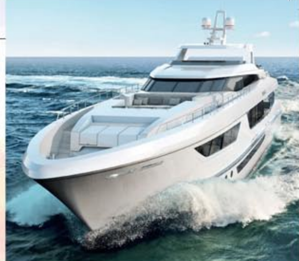
External views of Nina, digital renderings. Note the sign of the horizontal bridge on the upper deck and the semi-displacement hull.
